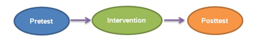
A pre-test/post-test design is an experiment where measurements are taken both before and after a intervention.
